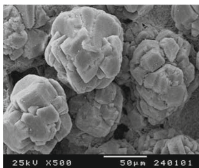
Fig. 4 SEM images of \text{Al}_2\text{O}_3 particles
