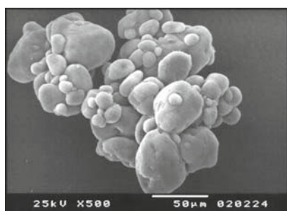
Fig. 5 SEM images of \text{RDX}_{\text{ph}} particles
